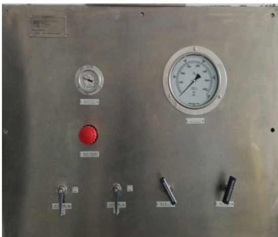
PIC6. Pneumatic hydrostatic test system(250MPa)
